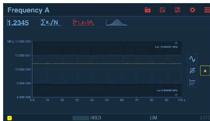
Figure 2: FTR-210R has built-in continuous comparison between the GNSS-receiver and the internal oscillator. The frequency offset is displayed and stored and a traceable calibration protocol can be produced at any time.
