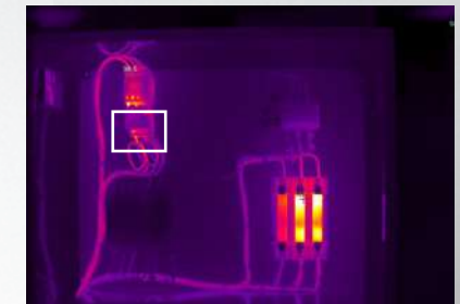
Full image, taken from 5 feet away with a TiX1000 infrared camera. The area shown in the white box is blown up below.
