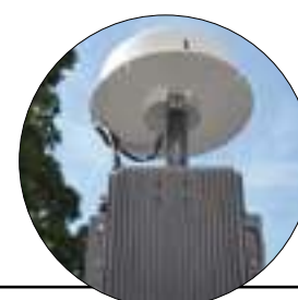
STATION CHARLIE (fixed installation): ▶ SignalShark Outdoor Unit ▶ ADFA ▶ LTE modem ▶ Software: Decodio ReX
