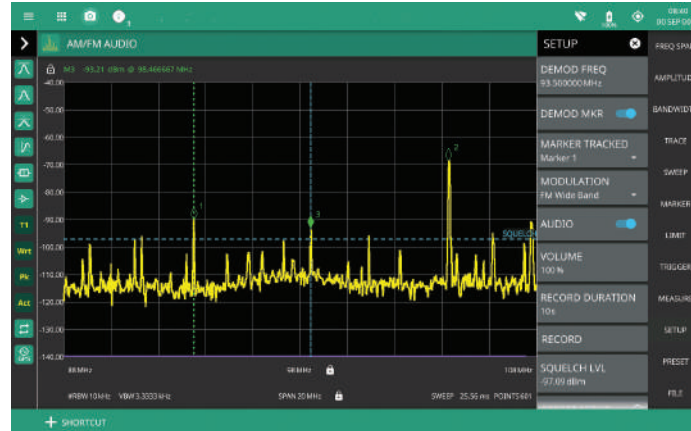
AM/FM Signal Demodulation at Marker Frequency
