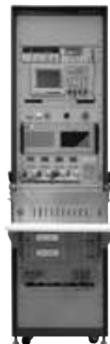
DC to DC Converter ATS
