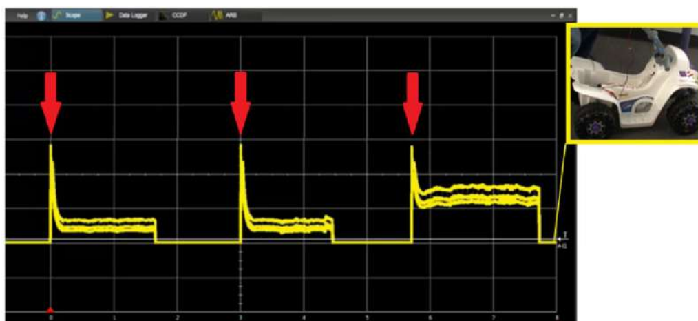
Figure 3. Example of a typical peak power surge waveform. The start-up current spikes as indicated by the red arrows each time the acceleration pedal on a toy electric vehicle (figure subset) is applied.
